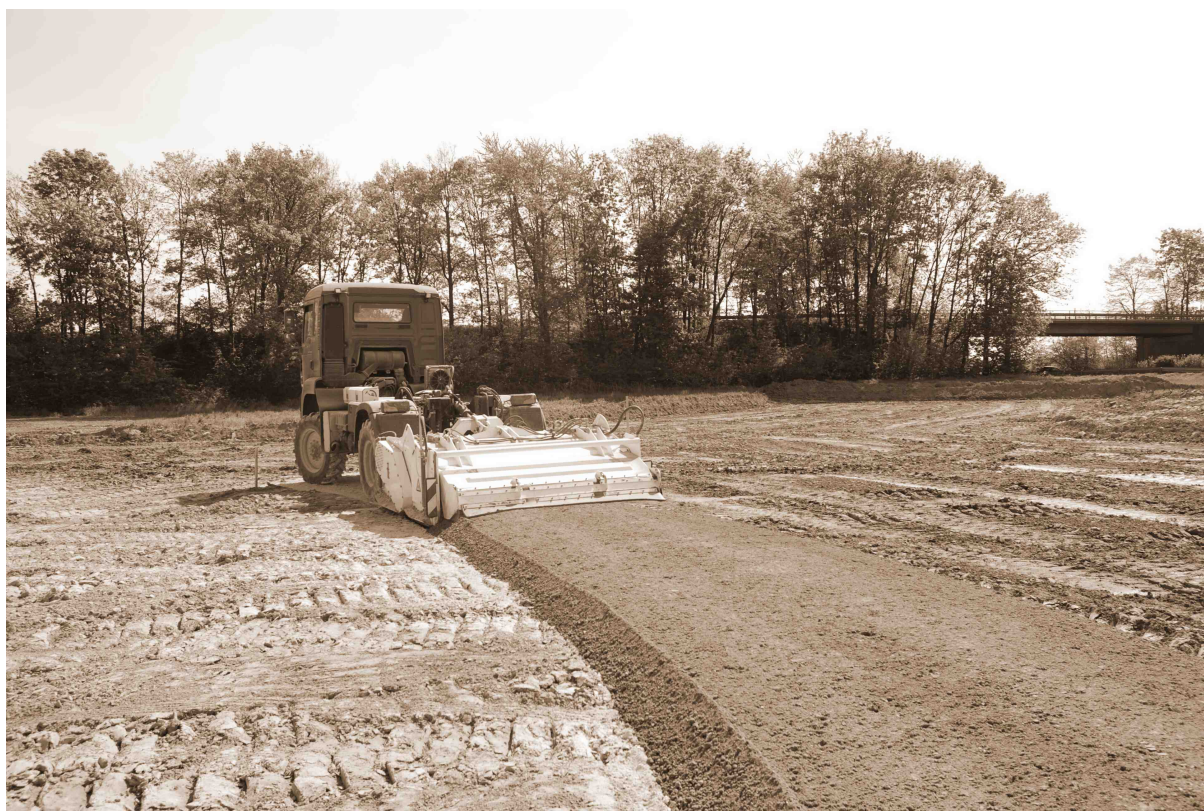
Extremely expanded tires (up to 710 mm) and 4-wheel-drive / differential lock provide for best traction on difficult grounds.
