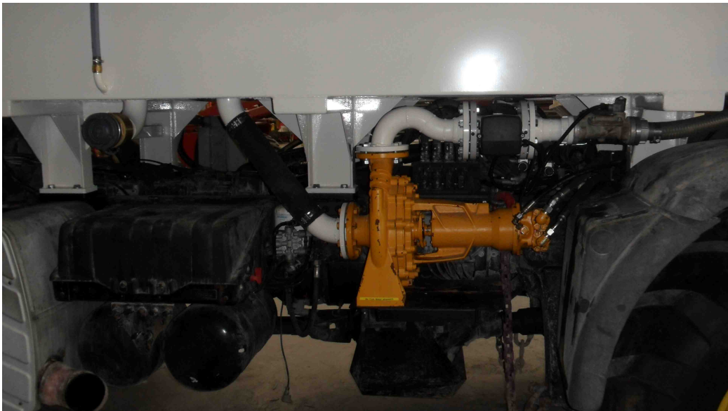
installation of the pump with digital flow-meters for a precise injection into the mixing room.
