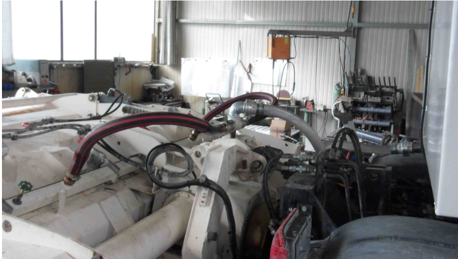
sealable fuel injection with flow-meter and exact dosage.
