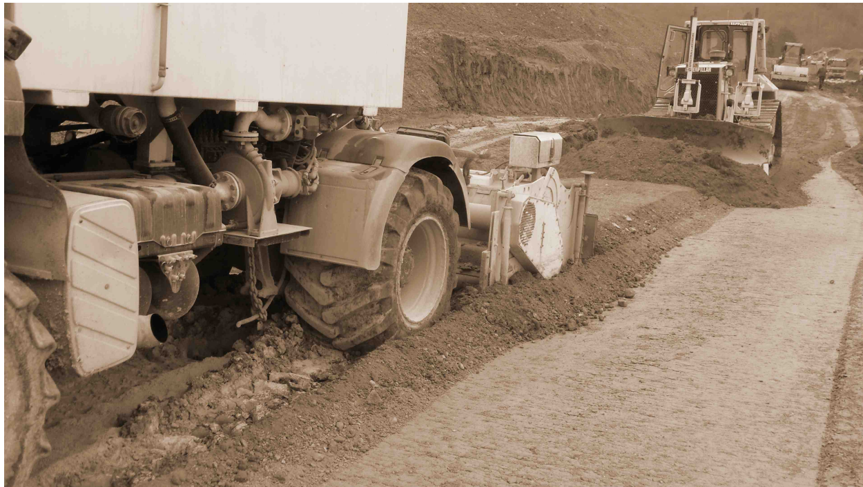
Extremely expanded tires (up to 710 mm) and 4-wheel-drive / differential lock provide for best traction on difficult grounds.
